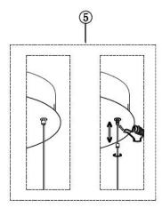
**Note:** Press the wire restraint to adjust the desired length of cable.
